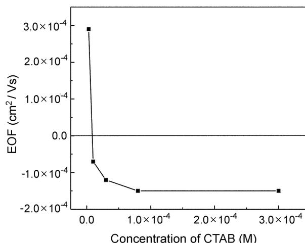
**Figure 1.** EOF as a function of CTAB concentration. Applied Voltage, 500 V; channel length, 4.0 cm, width, 80  $\mu\text{m}$ , depth, 20  $\mu\text{m}$ . EOF was measured by the current-monitoring method. Two different concentrations of TB buffer were employed for the determination of EOF.
